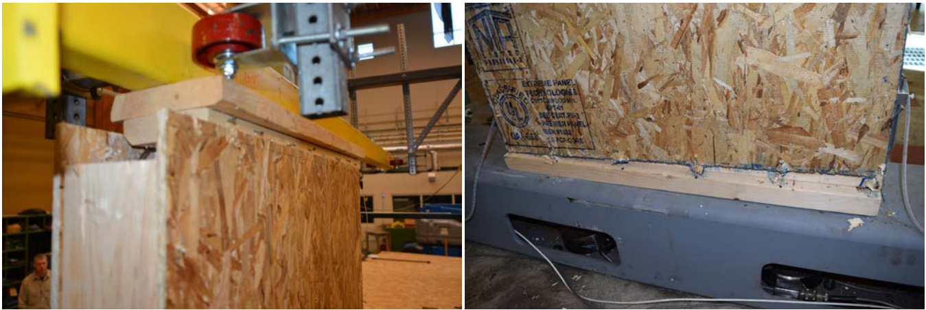
Figure 9. Failure modes for single-panel SIP tests.
